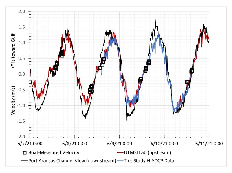
FIGURE 6. COMPARISON OF ADCP CURRENT PROFILE MEASUREMENTS WITH NEARBY SITES
