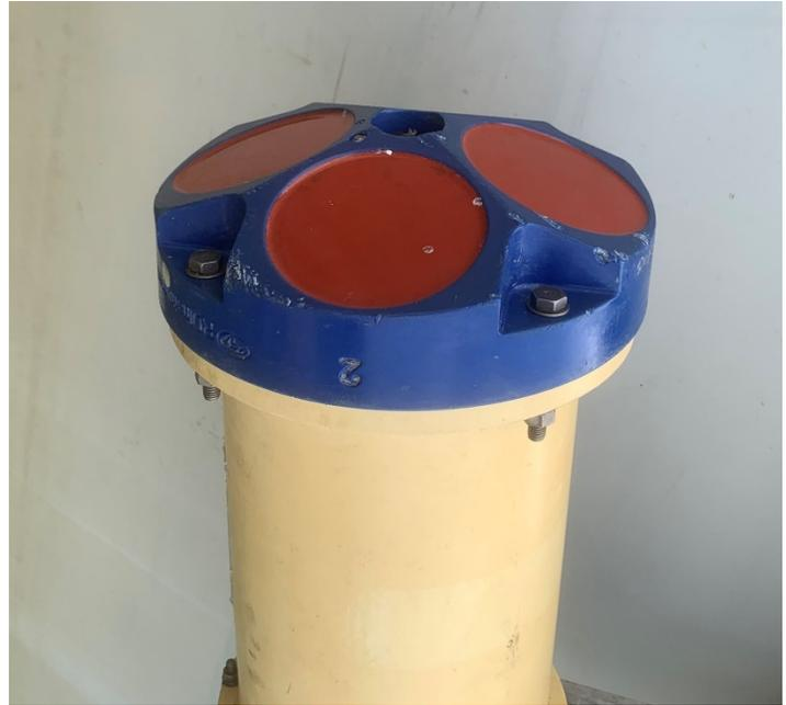
FIGURE 3. BOAT-MOUNTED (DOWN-LOOKING) ADCP
