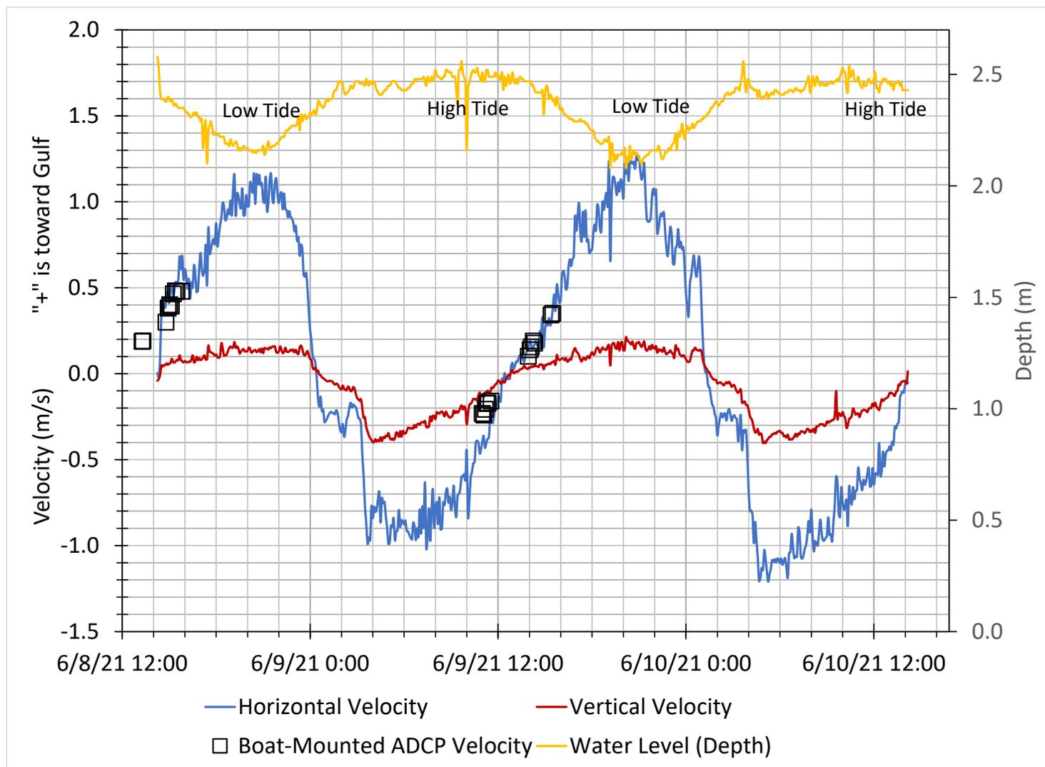
FIGURE 5. ACOUSTIC DOPPLER CURRENT PROFILER MEASUREMENTS
