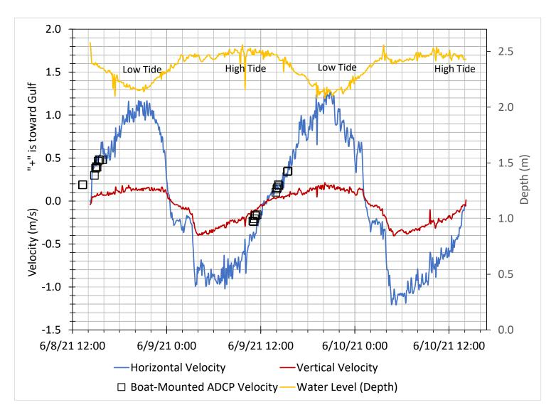
FIGURE 5. ACOUSTIC DOPPLER CURRENT PROFILER MEASUREMENTS
