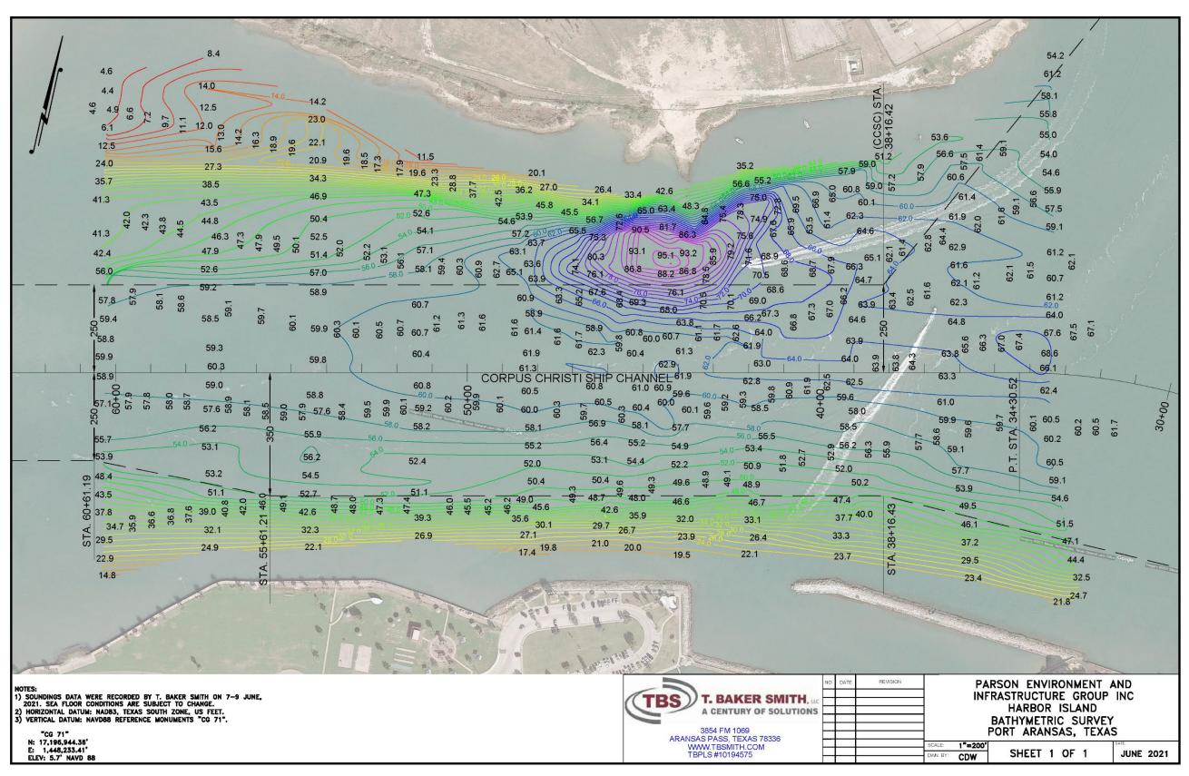
FIGURE 4. MEASURED BATHYMETRY
