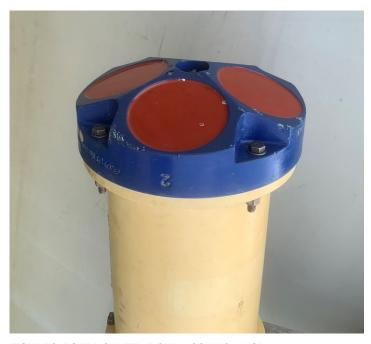
FIGURE 3. BOAT-MOUNTED (DOWN-LOOKING) ADCP
