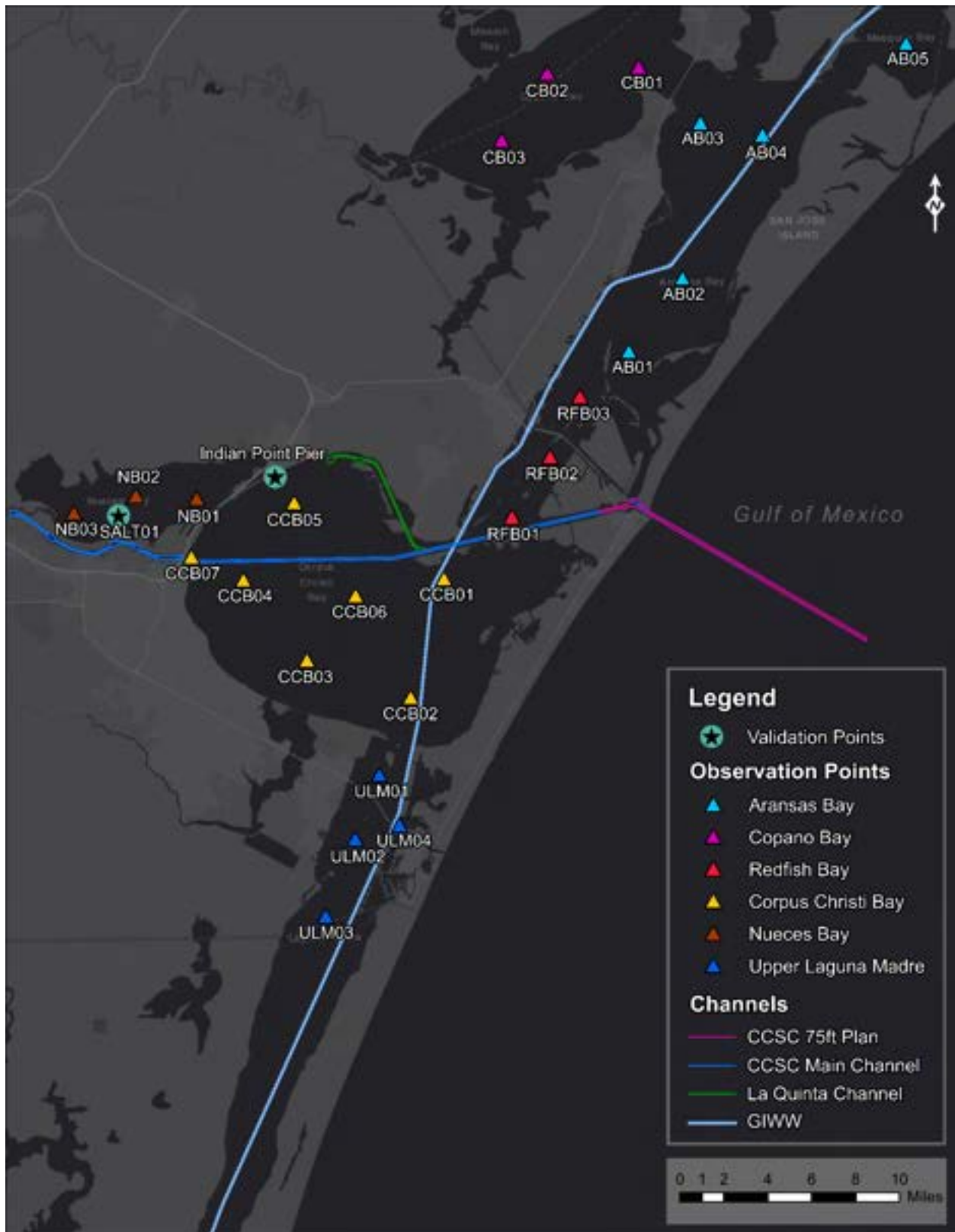
Figure 35. Validation points (Indian Point Pier and SALT01 in Nueces Bay) used for the surface salinity validation and model observation points used for three channel configurations comparison.
