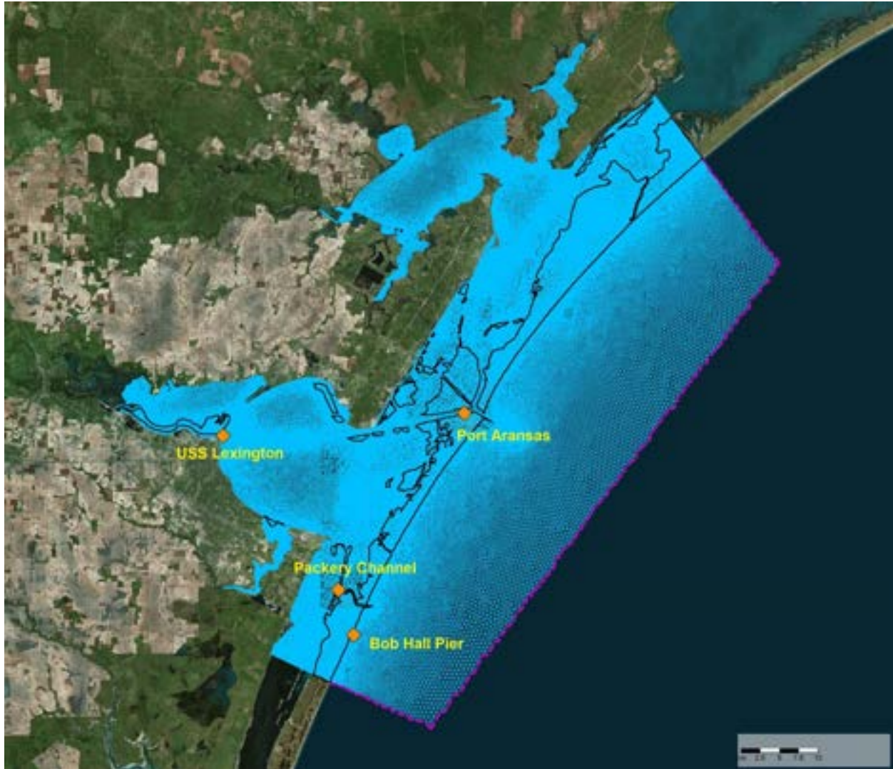
Figure 18. Delft3D-FM model grid is shown in blue. The magenta color shows the offshore boundaries and the black colored polygons show the land boundaries. The orange diamonds show NOAA tide stations used for input to the model (Bob Hall Pier) and water level output validation (Packery Channel, Port Aransas, and USS Lexington).
