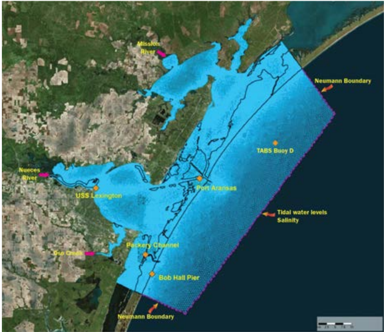
Figure 34. Delft3D-FM model grid is shown in blue. The magenta color shows the offshore boundaries, and the black colored polygons show the land boundaries. The model is driven with tidal water levels from Bob Hall Pier, surface salinity from Buoy D, and river flows from Oso Creek, Nueces River and Mission River (shown with pink arrows).
