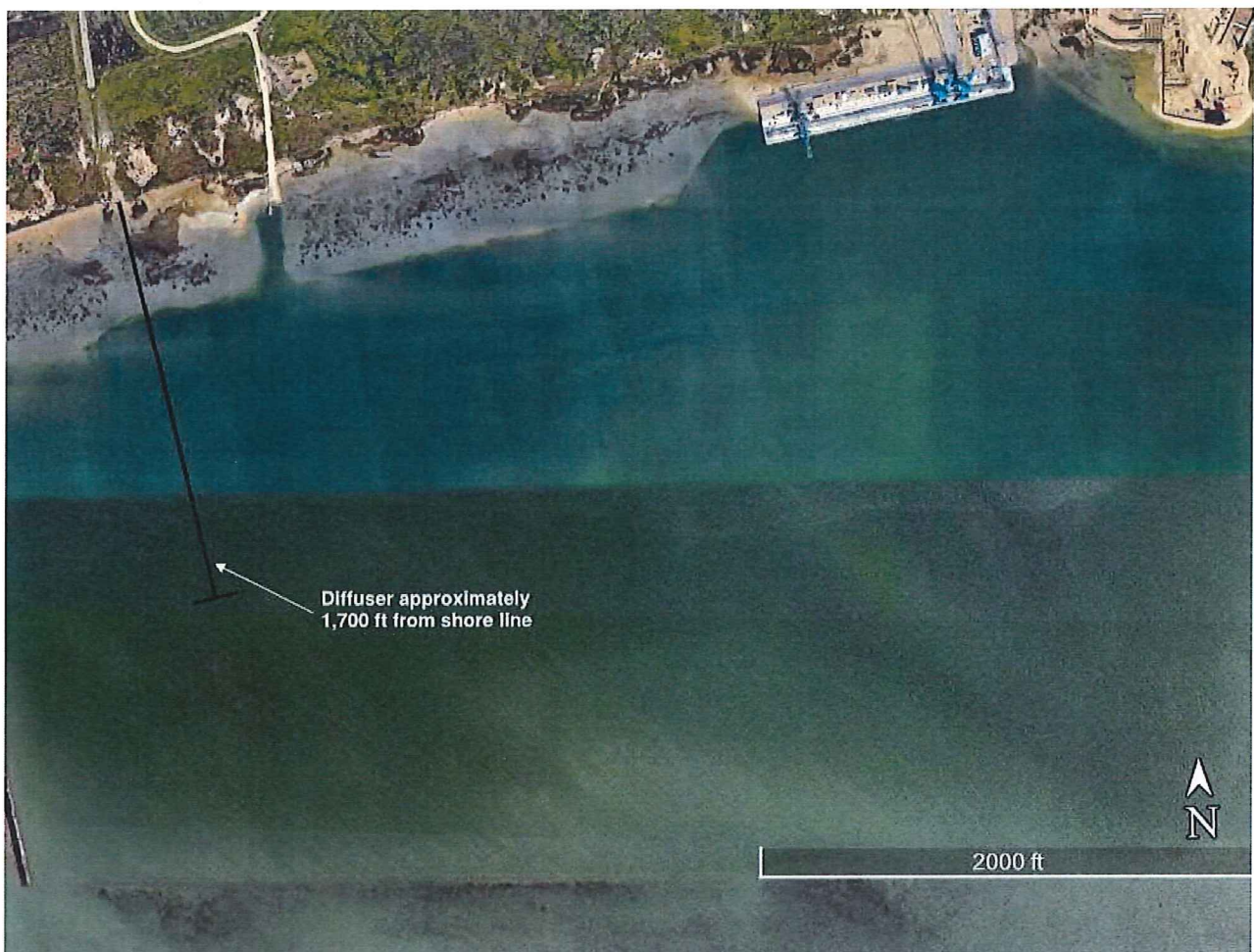
Figure 4 – Proposed Location for La Quinta Facility Diffuser
