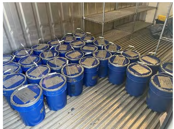
Photo 12 View of sediment samples stored in refrigerated unit at Martin Energy facility at or below 4°C.
