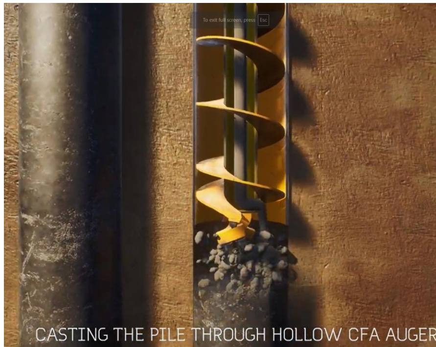
Figure 17. Casting Concrete Through Auger During Withdrawal 3
